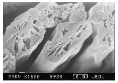
Figure 3. : SEM photos of DBC Fibres (solvent-ethanol); cross-section
